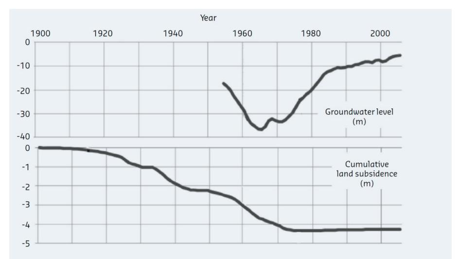
Figure 6. Land subsidence and groundwater level in Tokyo area (Kaneko & Toyota, 2011)
